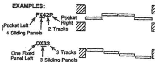
**SPECIAL APPLICATIONS** - Multiple sliding panels, pocket, or surface mounted installations, interior sliding partitions and other special design may be furnished. Not recommended for exterior use where door must be water-tight.
