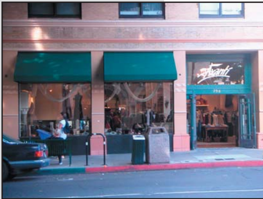
AWNINGS SHALL BE PLACED WITHIN VERTICAL ELEMENTS WHEN THE FACADE OF THE BUILDING IS DIVIDED INTO DISTINCT STRUCTURAL BAYS.
