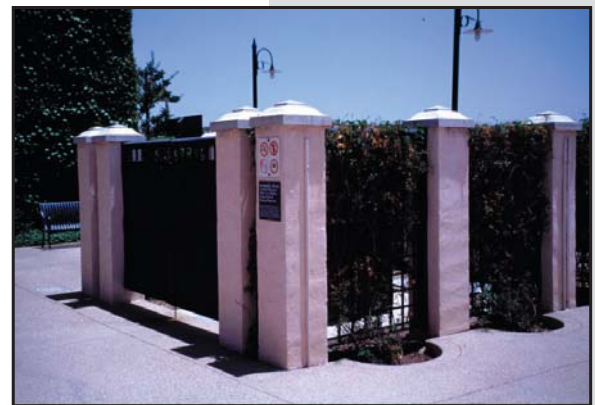
TRASH ENCLOSURES CAN BE SCREENED IN A VARIETY OF WAYS. THIS ENCLOSURE IS SCREENED WITH A FENCE, WALL, AND LANDSCAPING COMBINATION.
