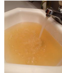
Figure 3. ORP affects metals stability and can cause discolored tap water (photo source: Hill & Friedman et al., 2010)
